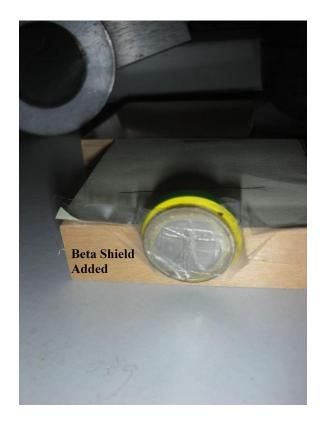
Then the source is taped to the end of a wooden block, this becomes the jig which holds everything stable while we change reflectors.
