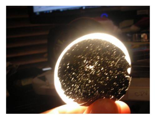
At sea level the mica is slightly bowed inwards due to the reduced pressure of the neon + chlorine gas inside. At higher altitudes, the mica flexes, and at about 8000 feet of altitude or equivalent air pressure, the bow reverses from concave to convex (Passenger airplanes are pressurized to 8000 ft equiv).
