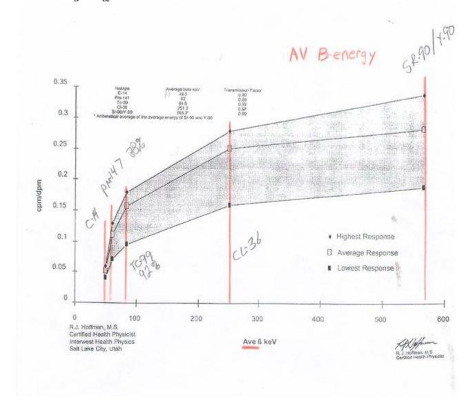
Without a calibrated source to compare against, any reading of a known energy beta emitter can only be accurate to a certain extent because of probe inconsistencies.
