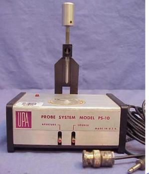
The radioactive source is Pm-147, a beta emitter of 0.2447 MeV (244.7 keV) Peak/ 0.0619 (61.9 keV) keV average at 99.99% probability and a T/2 (Half-Life) of 2.623 years. For the rest of this discussion series we will use the convention of keV for energy and refer only to the average beta energy.
