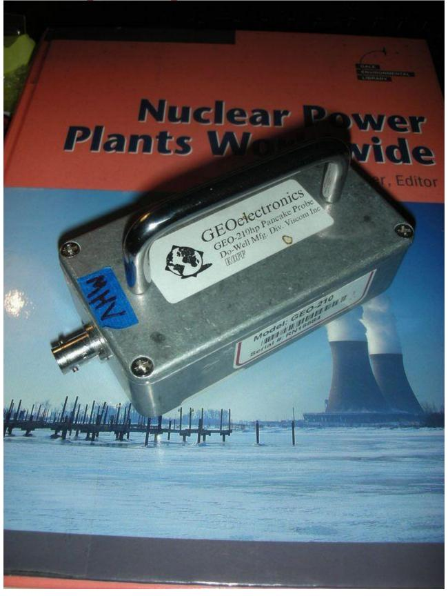
Pancake probe efficiency as beta detector is a variable depending on several parameters.
