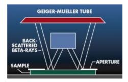
Some industrial systems use this same technique on a paint or coating production line to keep tabs on the coating thickness in real time, actually adjusting the machinery to keep it within tolerance.
