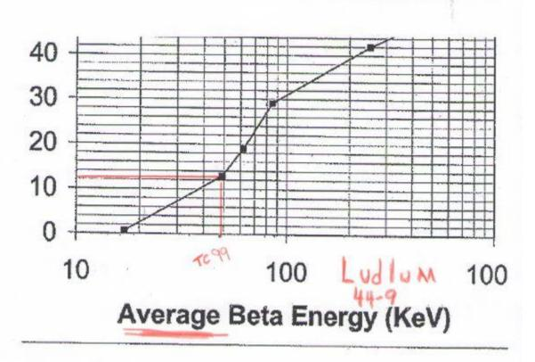
Hoffman's chart is probably more realistic, indicated the spread between actual tests made with different pancake probes and based on average energy:
