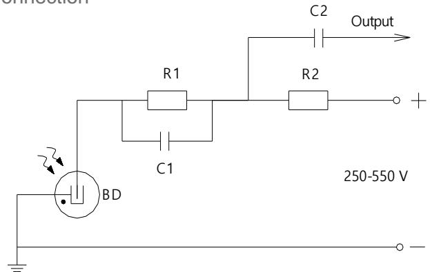
$$\begin{aligned} R1 &= 7.0 - 10.0 \text{ M}\Omega & C1 &= 3 - 5 \text{ pF} \\ R2 &= 2.0 - 3.0 \text{ M}\Omega & C2 &= 7 - 15 \text{ pF} \end{aligned}$$
