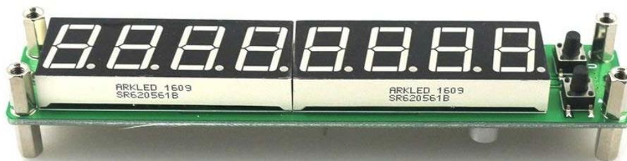
Frequenzimetro 100 kHz – 1GHz
