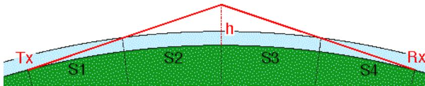
**Fig. 2.1.** Ionospheric single hop propagation.
