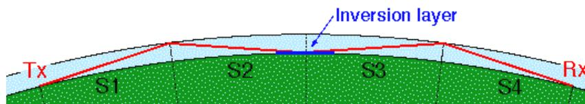
Fig. 6.14. Double hop propagation supported by an inversion layer.
