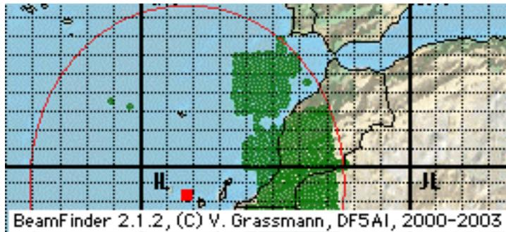
**Fig. 6.4.** Potential Sporadic E positions in single hop propagation.
