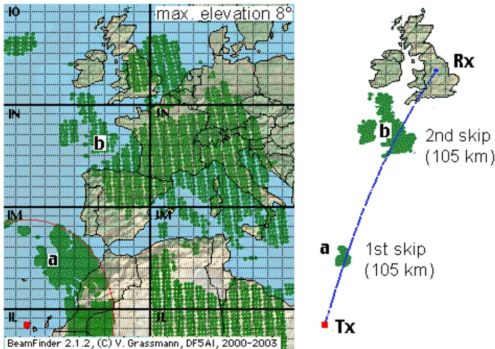
**Fig. 6.3.** Left: Potential Sporadic E positions in double hop propagation. The first Sporadic E cloud is always located within the red circle ( $0^\circ$  elevation). Right: Example of double hop propagation from the Canary Isles to central England.
