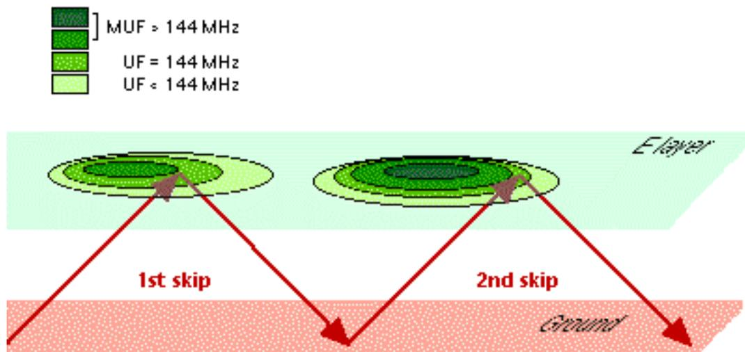
Fig. 6.13. Horizontal structure of Sporadic E clouds enabling double hop propagation.
