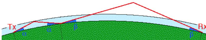
**Fig. 6.12.** Double hop propagation assuming unequal skip lengths.
