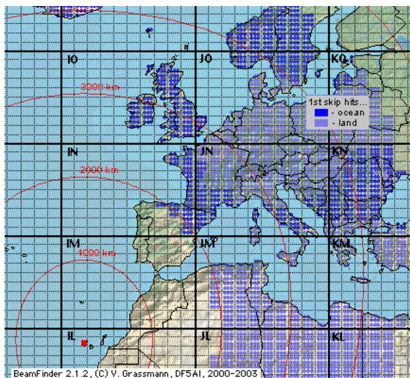
**Fig. 6.2.** Potential dx targets in double hop propagation (calculated for the IL18 grid square, maximum elevation 10°).
