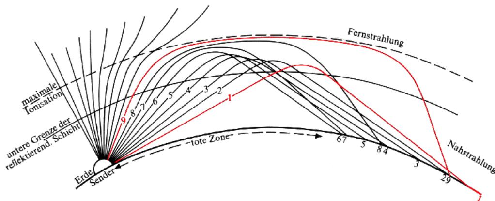
Fig. 3.2. Ray paths in ionospheric propagation [53].
