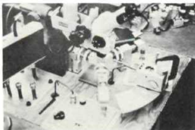
Fig. 11 — This figure shows the system in more detail. Apparent in the photograph is one of the phase shifters, bottom, the sampler on the left, a microscope at the top, a positioner for making contact to the transistor, right, and the three signal ports terminating in the transistor chip fixture in the center.
