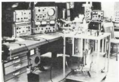
Fig. 10 — This is a photograph of the first system built to measure the three-port scattering parameters of transistor chips.
