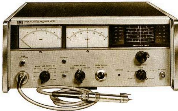
The HP Model 4815A RF Vector Impedance Meter covers the 500 kHz to 108 MHz frequency range. Measuring terminals are contained in a probe which may be used to make in-circuit measurements referenced to ground.
