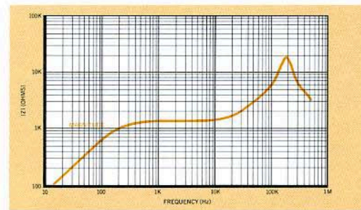
Fig. 13. Plot of impedance as a function of frequency for an iron-core audio transformer terminated in 8 ohms.
