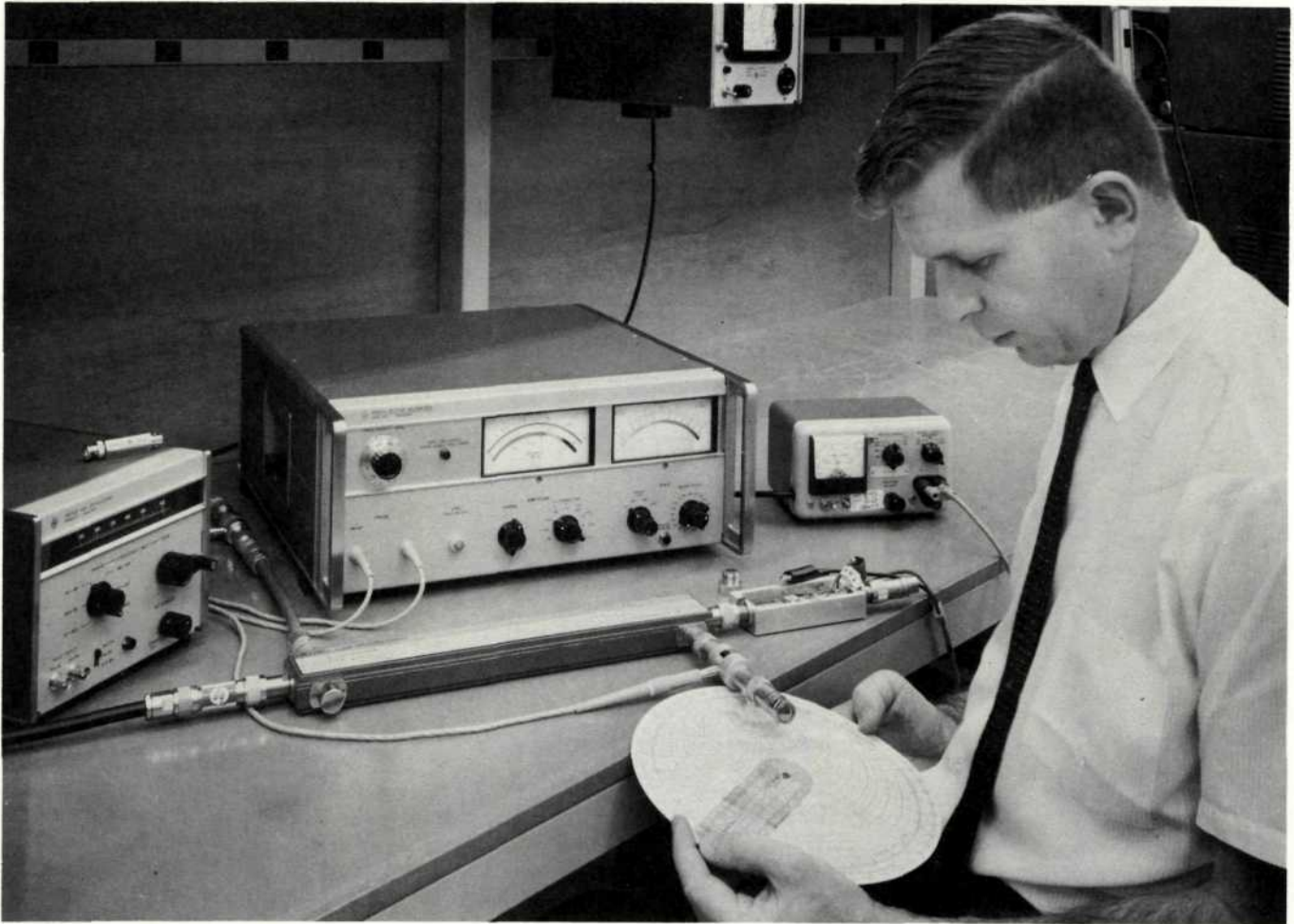
Figure 2. Measurement of Complex Input Impedance over 100 to 1000 MHz Range. Vector Voltmeter Amplitude and Phase Meter Readings Entered Directly on Smith Chart for Impedance Determination.
