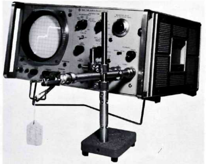
Figure 13. TDR Test of Transformer Subassembly
