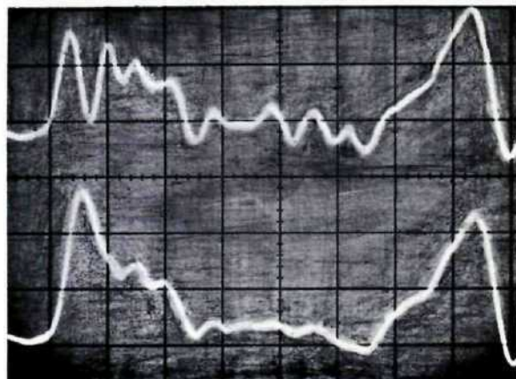
Figure 5. Moding Effects from Capacitive Tuning Screw (6 cm/cm of Display, \rho = .01/\text{cm} )
