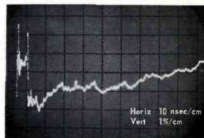
FIG. 12—Trace of cable shows construction irregularities and increasing series resistance.
