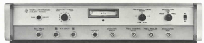
Figure 4. HP 8708A Synchronizer phase locks either HP 606B or 608F, giving dual range versatility in a single compact unit. Unique system provides automatic phase lock and continuous tunability for simple and flexible use.
