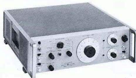
Figure 19. The \text{hp} Model 215A has a 50-ohm source impedance and delivers a 20 volt pulse into an open circuit. This instrument can be incorporated in a TDR system when extremely small resistive mismatches are to be measured.
