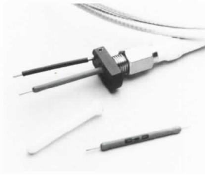
Figure 21. Transmission measurement using the HP 54006A 6 GHz probe
