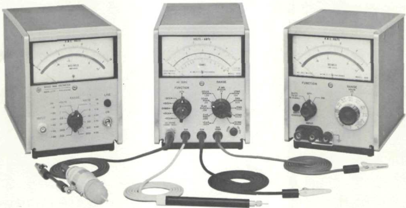
Hewlett-Packard AC voltmeters are manufactured in each of the three basic kinds, rms-responding, peak-responding, and average-responding. Illustrated is one example of each: Model 3400A rms-responding (left), Model 410C peak-responding (center), and Model 403B average-responding (right).
