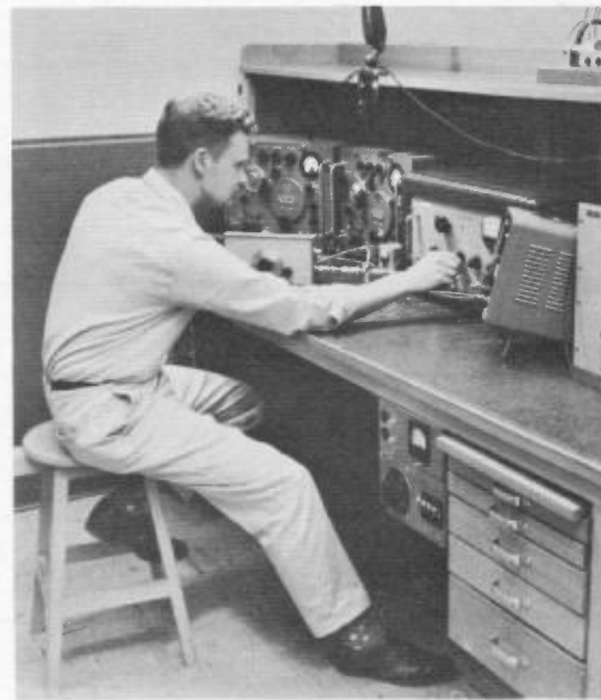
Ted Thomsen, a development engineer with the -hp- Standards Department, is shown checking the calibration of a 393A Variable Attenuator at one of the microwave test benches.
