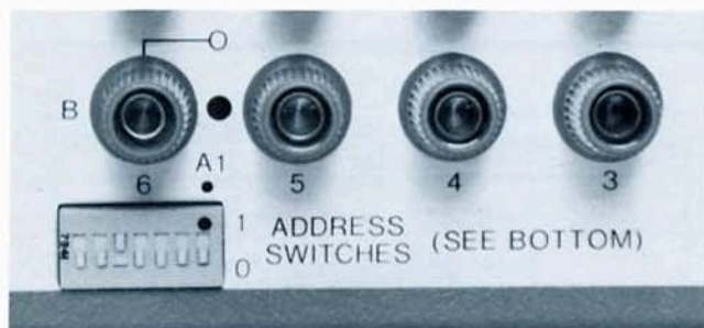
Figure 4. 59306 address switch settings.
