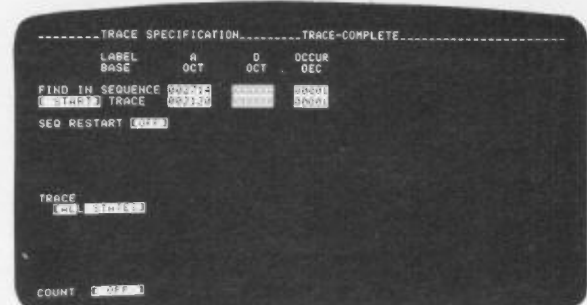
Figure 20. Trace specification for capturing the interrupt message output routine following entry from path A, (figure 19) which includes an address, 2714g, which is unique to path A.
