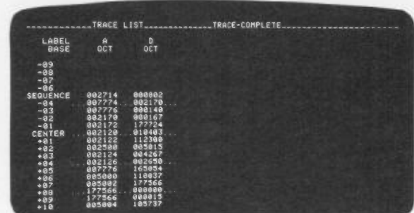
Figure 21. Changing the Trace Specification menu of figure 20 to CENTER trace mode produces a trace list which shows that four states occurred between the two sequential trigger words, addresses 2714g and 2120g.
