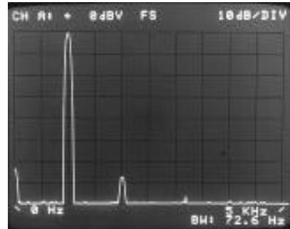
Figure 4.2 Powerline sidebands of an Audio Oscillator - Band Selectable Analysis and Hanning window used for maximum resolution.
