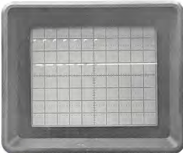
Figure 4. Single-shot stored display of seven control pulses generated by a write to output port instruction. This display was externally triggered by a Logic State Analyzer at instruction 0CF5_{16} as shown in figure 3.
