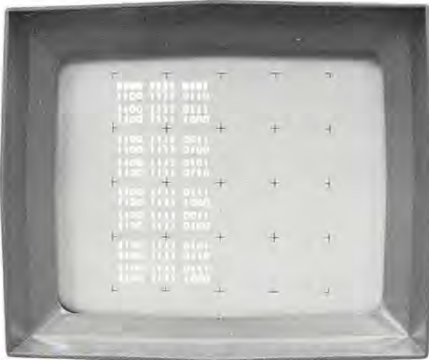
Figure 3. Logic State Analyzer table display of program execution that generates seven control pulses.
