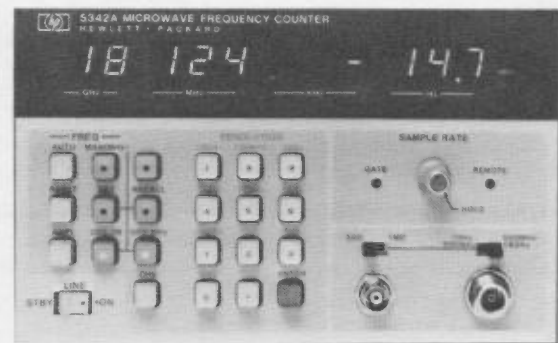
Fig. 1. Nine diagnostic modes are available with the counter in AUTO mode. The SET key is pushed twice and is followed by the appropriate digit key.
