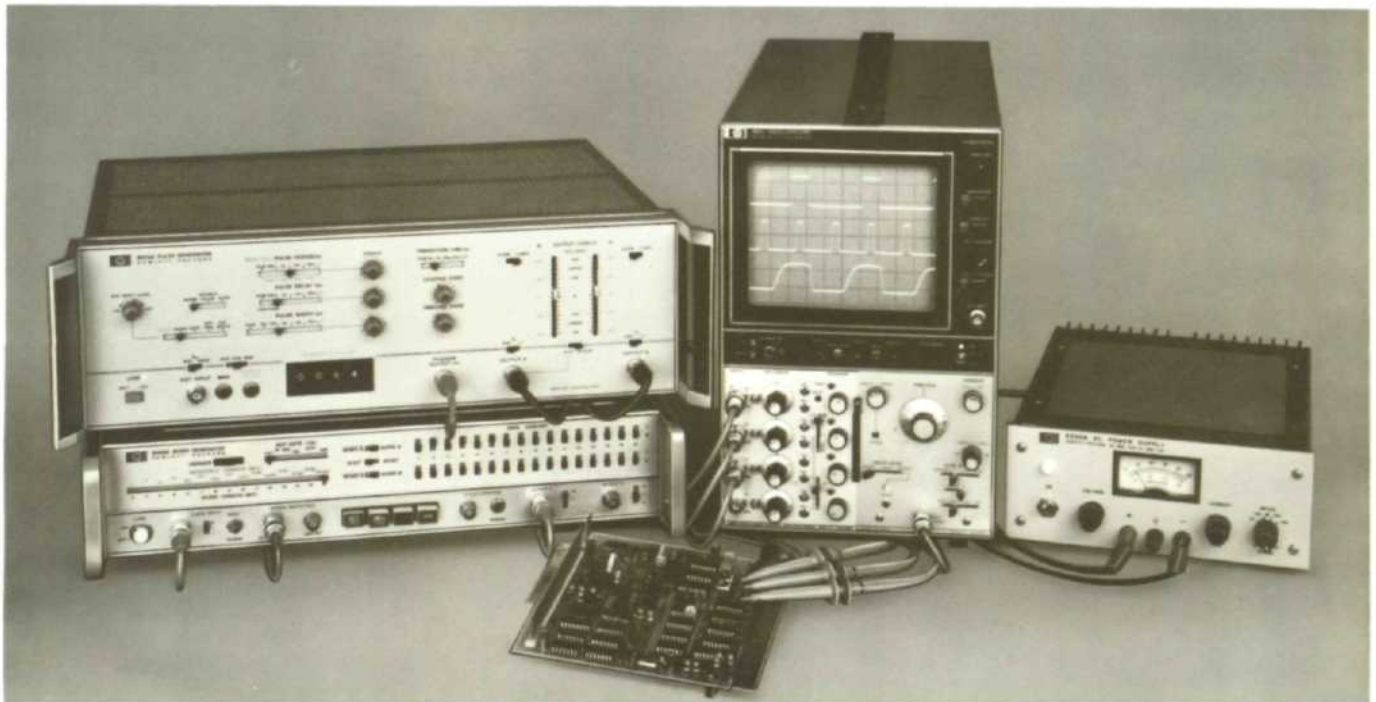
Figure 15. Photograph of Complete Parametric Test Set
