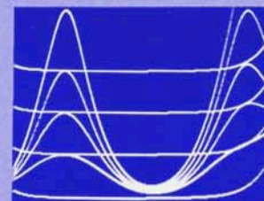
Figure 21. Equalizer peaking curve boost increments, at 100 Hz and 15 kHz center frequencies. Expanded scale 1 dB/vertical cm with calibration lines at 2 dB intervals log sweep, 20 Hz to 43 kHz.
