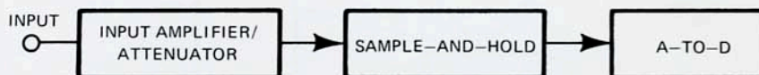
Figure 6-1. Sample-and-hold is located before the A-to-D converter but following the input amplifier/attenuator.
