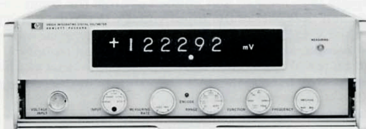
The -hp- 2402A uses the integrating-interpolation technique to achieve 43 readings per second with 5-digit resolution. Effective common-mode rejection exceeds 168 dB at 60 Hz \pm 0.15%. The high effective CMR is a result of integration and guarding.
