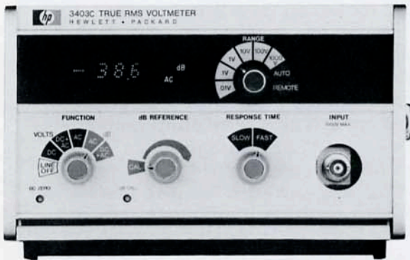
The -hp- 3403C uses a thermopile to make true rms measurements from 2 Hz to 100 MHz. This 3-digit DVM has ac ranges from 10 mV full scale to 1000 V full scale. AC accuracy equals \pm 0.4\% mid-band for 90 days. Crest factor equals 10:1 at frequencies > 25 Hz.
