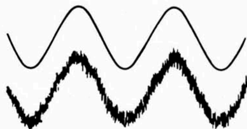
Figure 26. Phase measurements of noisy signals are readily made with the new 3575A Gain-Phase Meter. Even the high-frequency noise present on the lower trace does not preclude a useful phase measurement, for it only results in a phase offset of 2.50° and the measurement is free of jitter or bobble in the readout.
