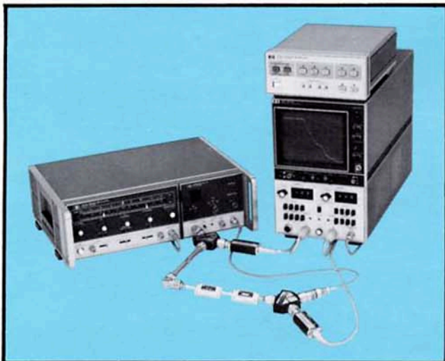
Figure 1. 105 dB Dynamic Range Measurement with the 8755.
