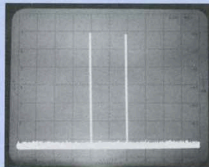
Figure 20B. Spectrum Analyzer display of two large signals after Pre-selector added. Log Ref: -10 dBm. Scan width: 50 MHz/div. Center frequency: 3.5 GHz.
