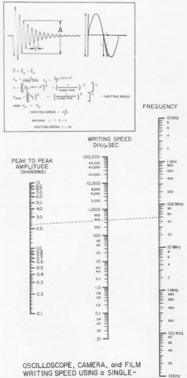
OSCILLOSCOPE, CAMERA, and FILM WRITING SPEED USING a SINGLE-SHOT DAMPED or UNDAMPED SINEWAVE
