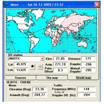
The Doppler offset calculated from the EME SYSTEM software is -206 Hz. This Doppler value has been confirmed from the experiment (-208 Hz detected). The sky noise temperature was 307 %, and the extra loss path -1,29 dB
