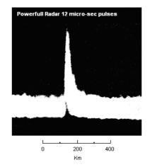
Fig.2 reflections observed from the moon employing a powerfull radar using 12 micro sec. pulses. The short range extent of the signal spectrum confirms that the reflections ae largely from the center of the visible disk. The Graph is taken from this document: "Radio communication via the Moon" by J.V Evans (COMSAT Laboratories-United States)
