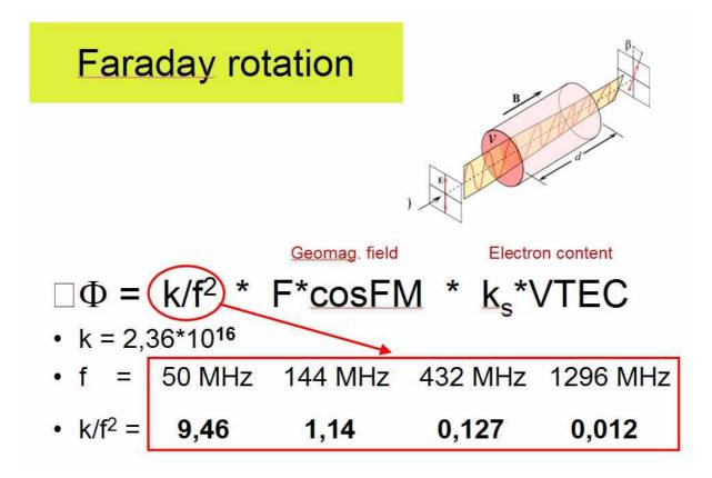
Faraday rotation is proportional to the magnetic field component and to the amount of plasma traversed. The formula gives the average rotation value, since the ionosphere is turbulent., which cause short term variations of plasma density.
