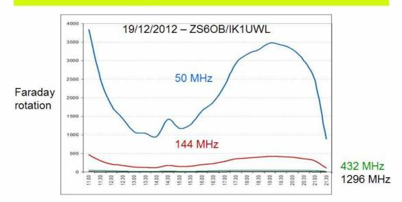
The K/f<sup>2</sup> coefficient determines rotations of thousands of degrees on 50 MHz; hundreds on 144, tens on 432, and is negligible on 1296 MHz and above.
