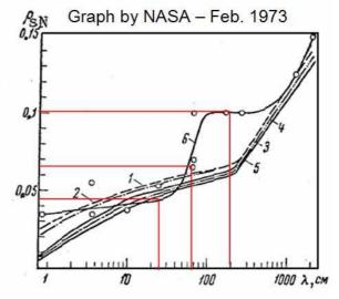
This is a graph of reflection coefficients from the above radar experiments. From which we gather that the amount reflected as a function of frequency is:
