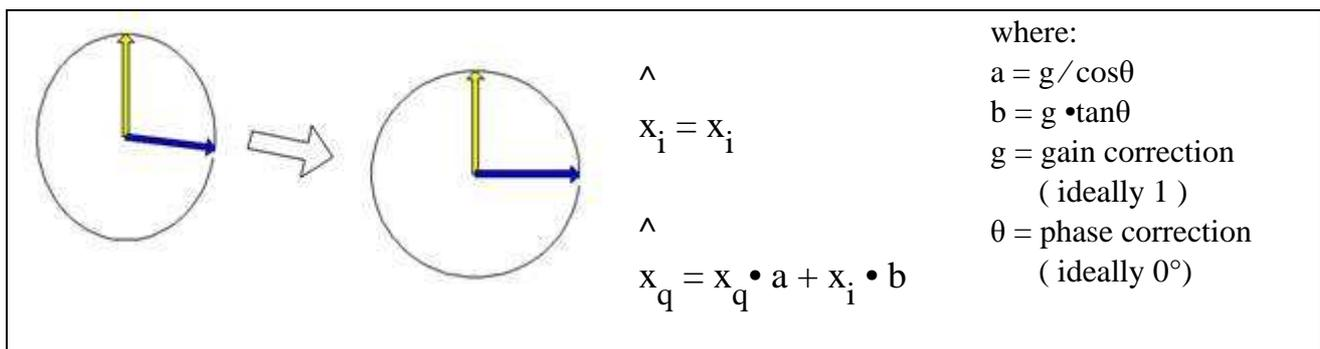
Fig.3 - Sample rotation and amplitude adjust.
