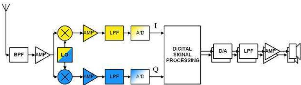
Fig 1- Direct down-conversion receiver
