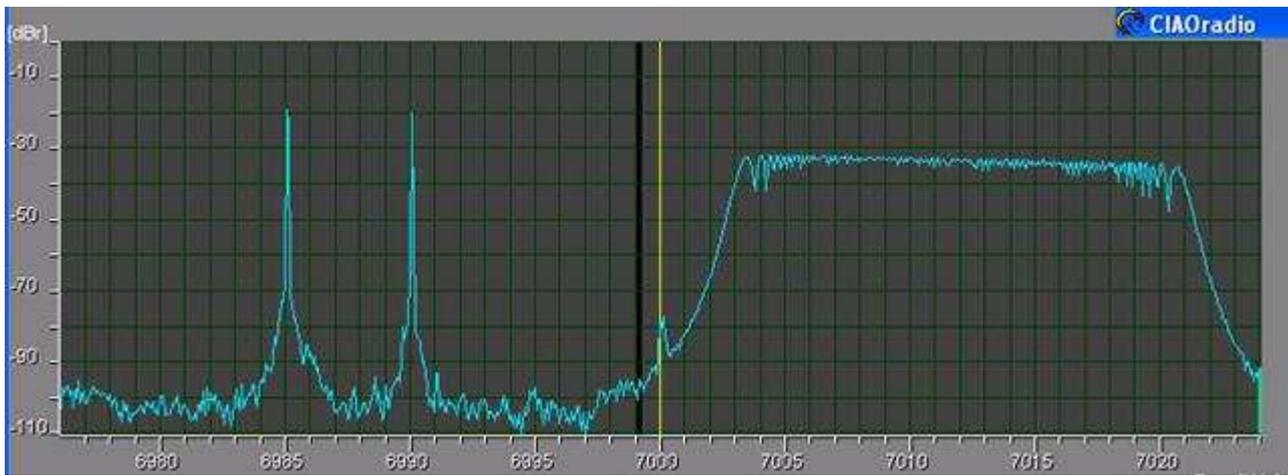
Fig.11 – CIAOradio output imbalance with AIQB (test signal 3)
