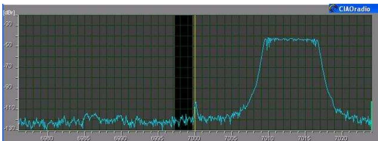
*Fig.9 – CIAOradio output imbalance with AIQB (test signal 2)*
