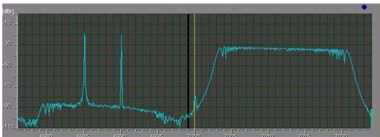
*Fig.10 – CIAOradio output imbalance (test signal 3)*
