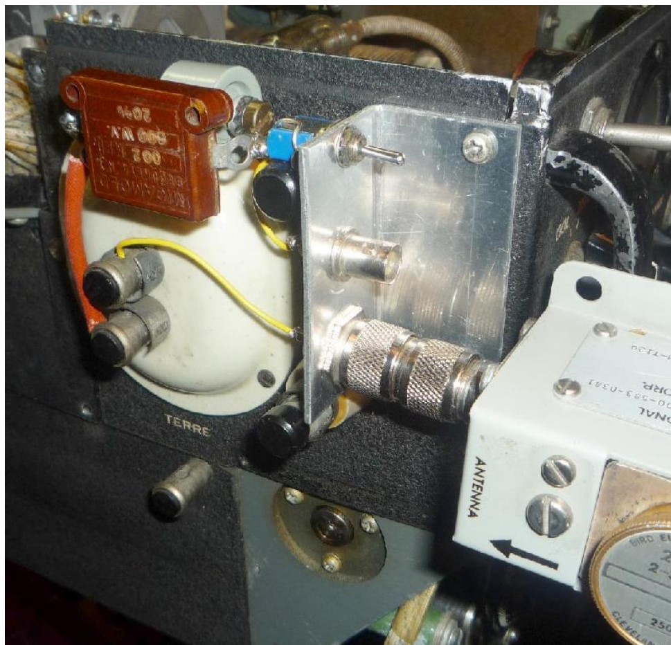
Figure 4.1 – ART-13 RF Connections
