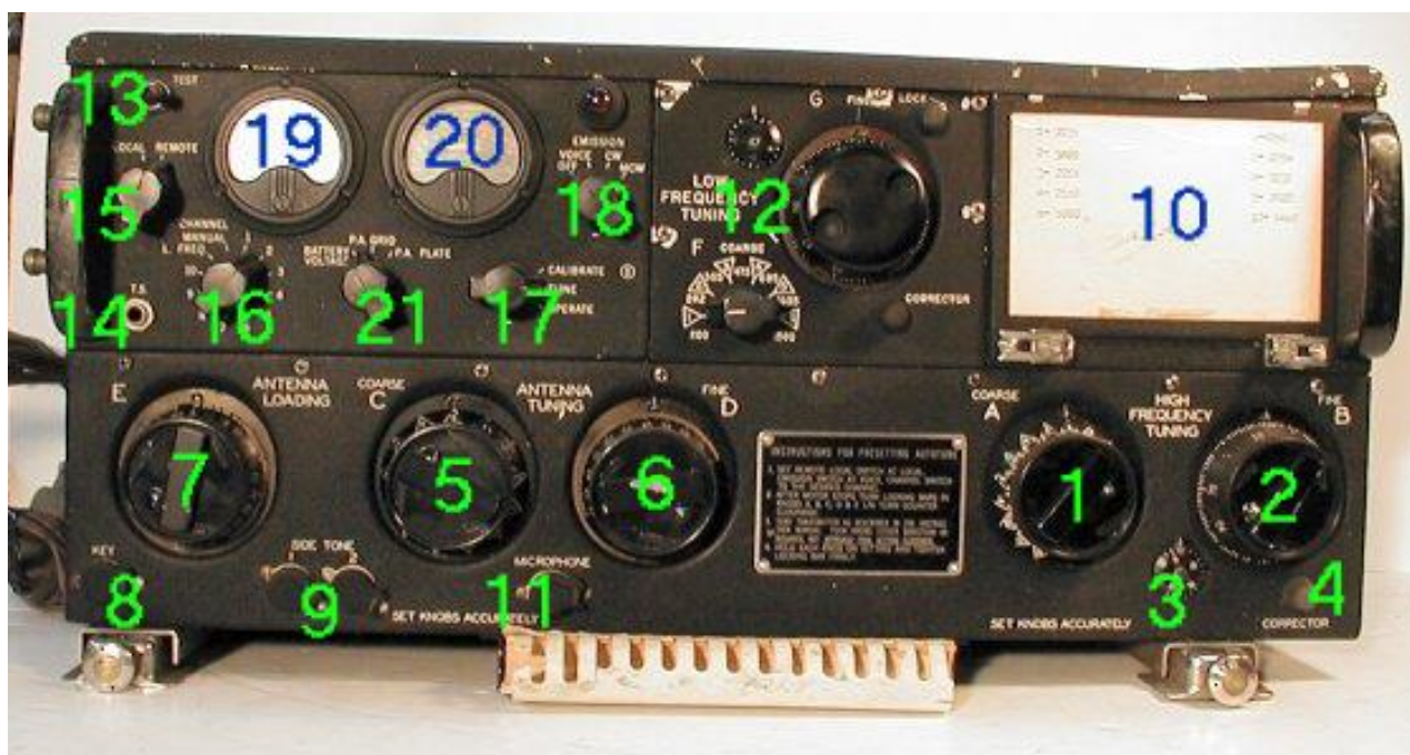
Figure 2.1 – ART-13 Front Panel
