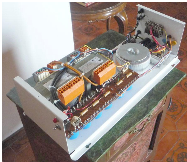
Figure 3.2 – ART-13 Home-Made AC Power Supply - Pictorial
