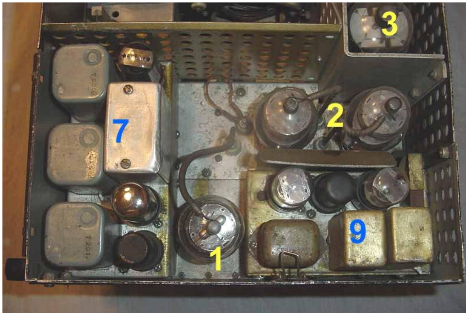
Figure 2.3 – ART-13 Audio, CFI, HFO and Frequency Multipliers Compartment
