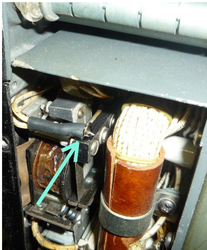
Figure 4.6 – Relay Harness Alterations
