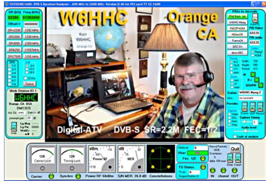
Screen-Shot of Tutuone analyser receiving DVB-S using ODROID
