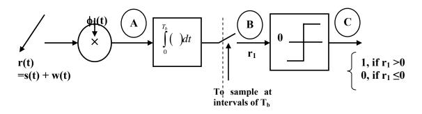
**Fig. 5.24.3** A scheme for coherent demodulation of BPSK modulated signal following the concept of optimum correlation receiver
