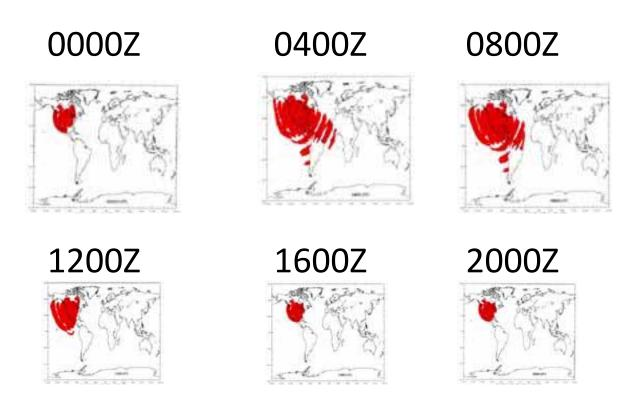
Red shows areas where signal levels of >= 100 microvolts/meter are present for the time shown.
