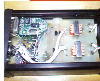
Fig. 7: The p.t.t./c.w. circuit and isolation transformer.
