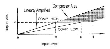
voice, whispering, small or loud. By the constant output level, you can extend the communication distance by using rated output power of transceiver without any loss. So, now it becomes common to use compressor amplifier between transceiver and microphone.
