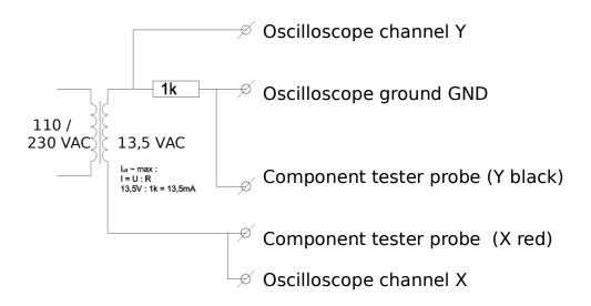
Connect the diagram above, set your oscilloscope to use X-Y function and invert channel Y. You can now use 'Component tester probe'-connections to test your components. On the following pages you can find some theory that can help you understand, the pages are from the Hameg HM504 user manual.
