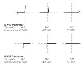
For a transistor the figures b-e and b-c are important. The figure e-c can vary; but a vertical line only shows short circuit condition.
