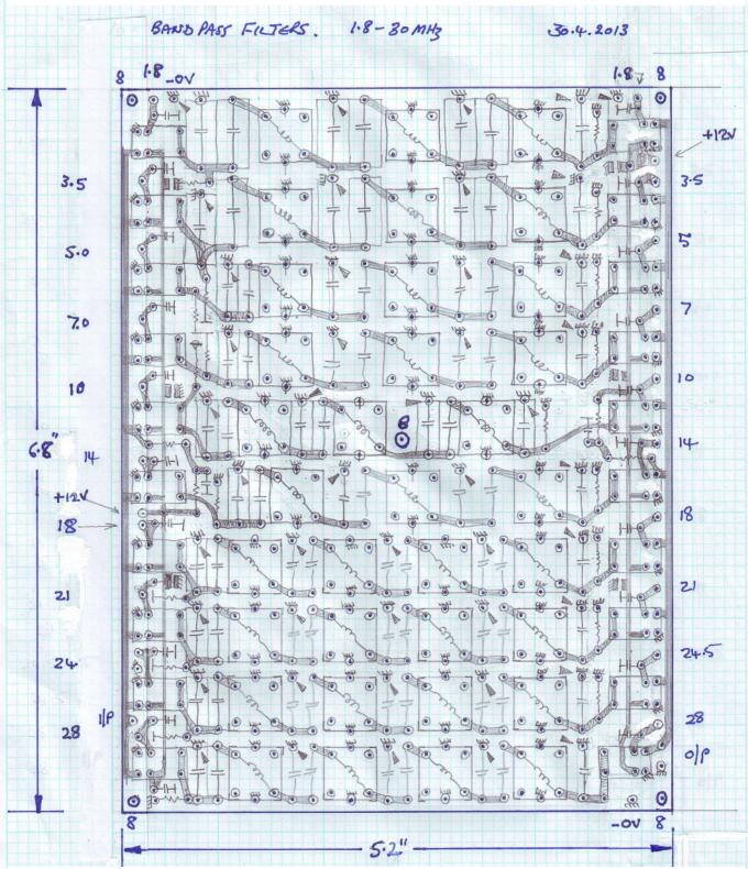
The above view is the solder side and all areas containing points marked as ground connections should be infilled with ground copper and connected through to the top copper groundplane.
