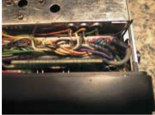
Figure 18 The position of the 3.3k resistors in the FT-790. The FT-290 is similar.
