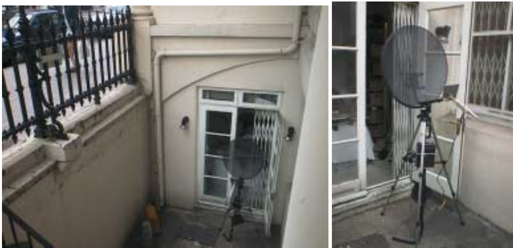
Figure 23 AO-40 reception at 8' below ground level
