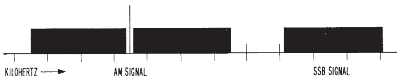
Figure 40. Relative spectrum space occupied by AM signal and SSB signal modulated by frequencies of 200 to 3000 Hz.
