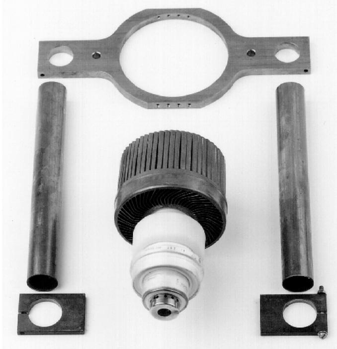
**Picture 9: Parts of the resonator (without Part R 2 und Part R 3)
