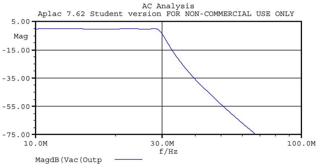
Due to the unprecise realisation with the real values, the attenuation of 0.5 dB is already reached at about 29 MHz.
