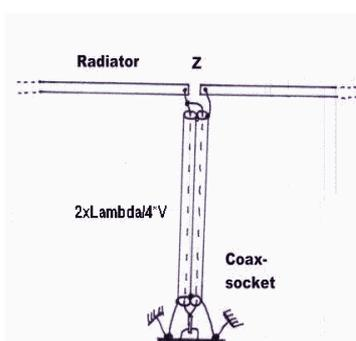
coax is affected by the velocity factor which depends on the dielectric material. Foam Coax have about 0.8 while PE has 0.67 !
