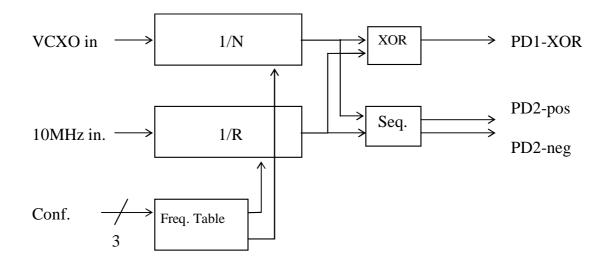
Fig 1 – Block diagram of the logic implemented inside the EPM3064.
