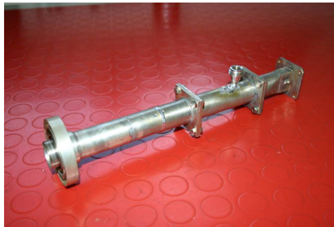
Figure 5- The circular feed assembly with choke rings positioned for an 0.3 f/D dish.
