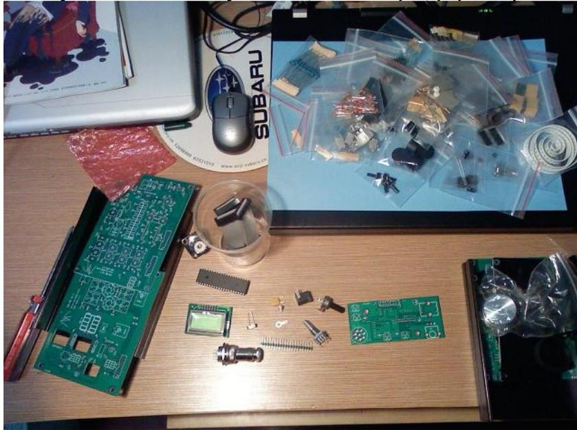
Start from the simplest board. I call it display and control board, or you can call it internal front panel, whatever you like. I haven't seen any part list posted yet, but you can easily figure out what to install by the printing on board. Solder two chip capacitors and SMD IC first on bottom layer (solder layer), and then the IDC connector. Pay attention to the orientation as shown.
