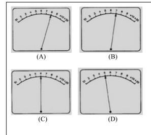
Figure 1 – I f a 1-kW signal pushes the S meter to S9, dropping to 250W will only to S8 (A). Drop to 62.5W and your down to S7 (B). Take the big downward leap to 15.6W and the meter reads S6 (C). Finally, dip to only 3.9W and the meter is S5 (D). So going from 1 kW to 3.9W only "cost" us four S units!
