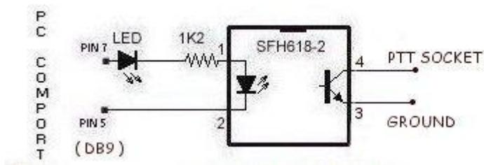
The RTS line is pin 7 and ground is pin 5 on the DB9 connector (pins 4 and 7 respectively on a DB25) .
