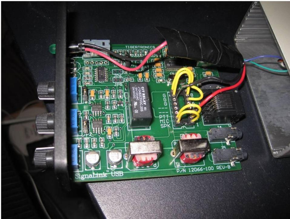
I drilled a hole for the new transmit LED in the front of the SignalLink box, and another hole in the back for the RS232 RTS signal (green and blue wires).
