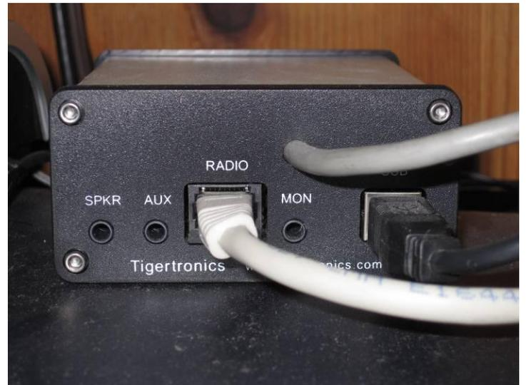
The Signalink has a built in VOX option that sends a PTT signal to the radio. This and the audio signals are in the cable connected to the "Radio" jack of the Signalink going to the radio's Accessory 2 jack on the back of the radio. (The large green LED on the front, and the grey cable on the back are modifications I'll talk about later.)
