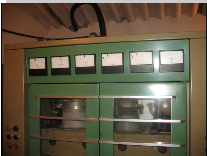
The Colombian built 5 Kw carrier (20 Kw PEP) output transmitter using two 4CX5000 for modulators.
