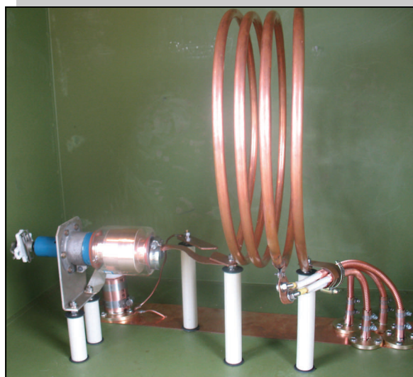
The 50 ohm in by four way 50 ohm out L/C match network at the array common point. The 0.50 inch copper tubing runs warm with greater than 10 amps carrier RF at 6.01 MHz.
