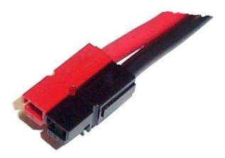
Put the connector housings together before putting the connector pins in, this is easier, especially when using heavy paired wire.
